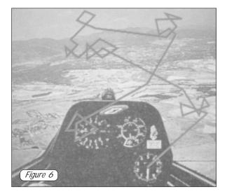
*The scanning eye movement of a beginner pilot Narrow sweep angle, spends too much time focusing on airfield (to right of instrument panel), village, clouds.*
