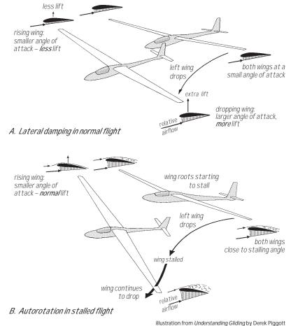
as autorotation and it is the cause of spinning (see Figure B). The autorotation combines now with the increased drag on the down-going wing and the reduced drag on the upper wing to produce a strong yawing motion to-ward the lower wing. At the same time the nose pitches down and the glider goes into a spin.
