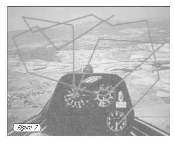
Scanning eye movement of an experienced pilot Wide sweeps along the horizon while keeping an eye on airfield location and all instruments.
