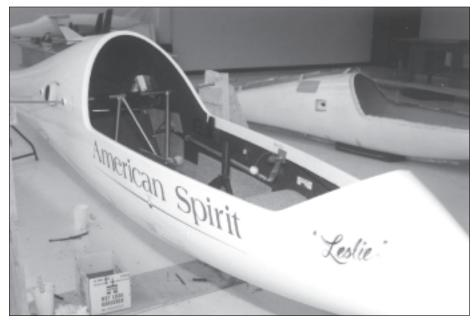
Fuselage shell has been joined here on the prototype Spirit.
