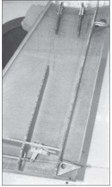
Right side of vertical stabilizer with honeycomb spars, control linkages, and rudder hinge supports being installed.
