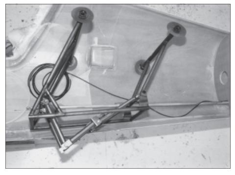
The steel tube frame tranfers the loads from the wings into the fuselage and down to the undercarriage. The frame will be glassed into the right half of the fuselage shell along with bulkheads, antenna coax shown here, controls, etc. before the shells are mated.
