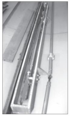
Honeycomb spoiler box, spoiler, and aileron linkage installed in the lower half of the wing. Note the carbon fibre shear web just to the left of the spoiler box.
