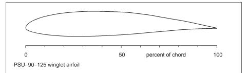
at negative  $C_{l}{\rm 's}$ , so that sideslips and horizontal gusts can be tolerated. The corners of the laminar bucket have been rounded to avoid unstable yawing moments that would be generated otherwise if the sailplane yawed to angles exceeding those corresponding to the sharp corners of the traditional Wortmann sailplane airfoils. Finally, the airfoil was designed to avoid laminar separation bubbles down to  $R_e=350,000.^{\prime\prime}$
