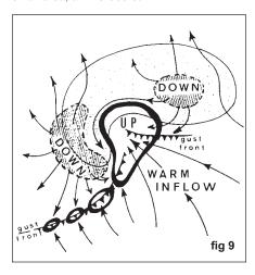
Figure 9 shows a plan view of a typical supercell. The heavy black line outlines the updraft. This is fed by the warm moist inflow that is shown entering from the southeast. The main area of precipitation at the surface is shown stippled. Two downdrafts are shaded in and the outward flow is indicated by curving arrows. The two gust fronts are shown by spiked lines. Notice that in the southwest quad-
