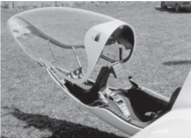
GLASFLÜGEL has recently been working on a project having the aim of completely redesigning the instrumentation and cockpit area of the modern sailplane. The company unveiled its "dream machine" which features a shallow cockpit pan cantilevered out from the main bulkhead, and a push-button instrument panel with all information appearing digitally on a "heads-up" transparent Liquid Crystal Display (LCD).
