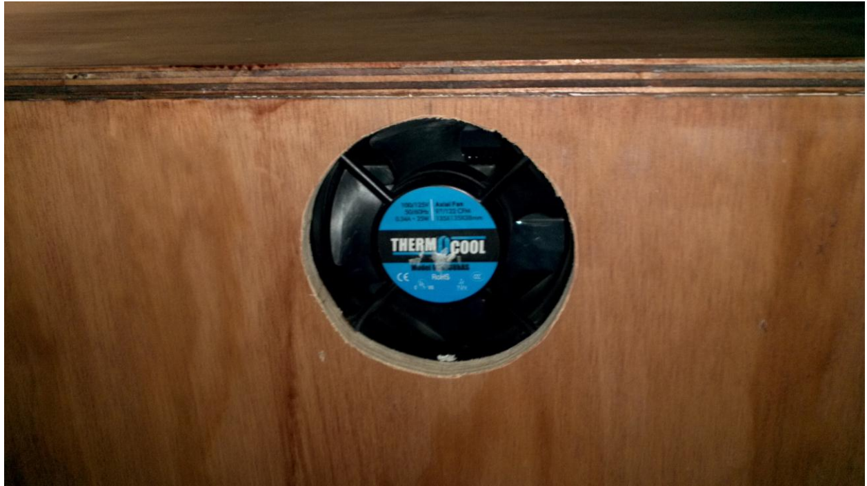
Back of cabinet mounted cooling fan – comes on when power bar surge protector is turned on
