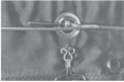
This pin is too far in. Note the thicker root of the pin could jam in the holder and make it difficult to pull the ripcord handle.
