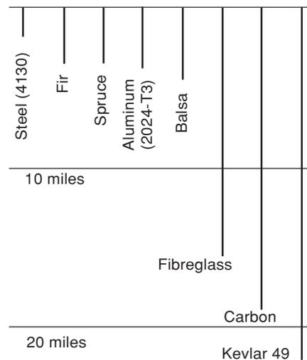
A comparison of different structural materials. Dividing the ultimate strength of the material (expressed in psi) by its density (expressed in lb/in<sup>3</sup>) gives an indication of the suitability of the material in aircraft construction. Each line represents the length of material (expressed in miles in the above graph) required to break in tension because of its own weight.
