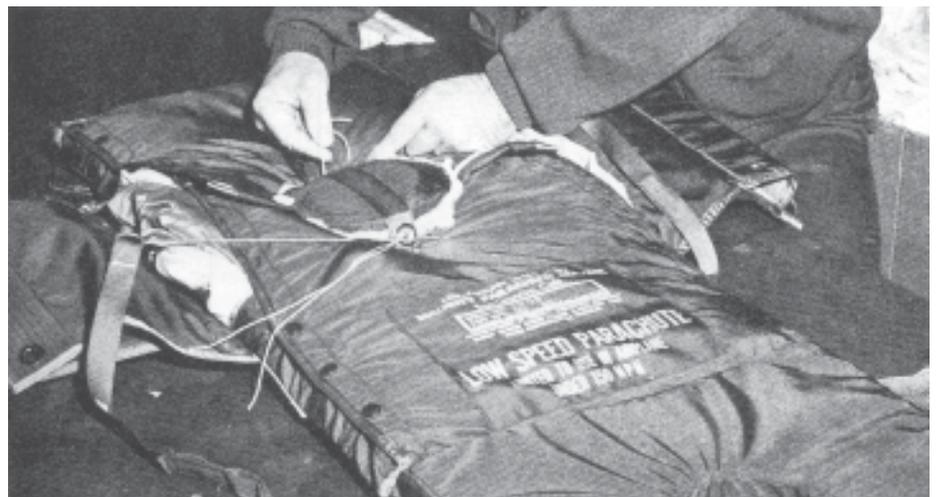
The pilot chute in this Security 150 (on the left) was placed UNDER the top and bottom canopy covering flaps rather than on top, the manufacturer's proper way of packing (shown above). As a result of this mistake, the pilot chute cocked itself sideways inside the container. When the
