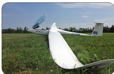
The HpH 304 “Shark”, the newest Czech design derived from the old Glasflügel Mosquito, features an advanced wing/winglet in 15/18m. There is also a jet sustainer version. Nick Bonnière readies for a launch at GGC.
