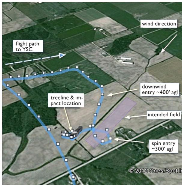
Accident occurred near the end of the convective day, thermals were broken up by wind, no attempt at thermaling below 1000 ft agl. Joined downwind at about 400 ft, initiated turn to final at 300 ft agl when a stall/spin developed. During the spin the glider impacted into trees, a branch entered the cockpit through the canopy.
