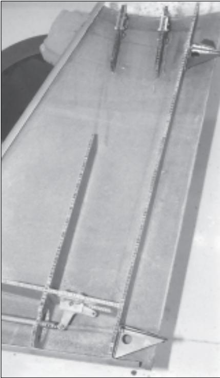
Right side of vertical stabilizer with honeycomb spars, control linkages, and rudder hinge supports being installed.
