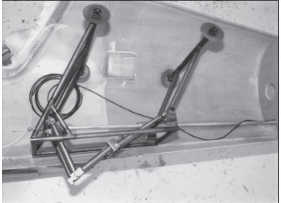
The steel tube frame transfers the loads from the wings into the fuselage and down to the undercarriage. The frame will be glassed into the right half of the fuselage shell along with bulkheads, antenna coax shown here, controls, etc. before the shells are mated.
