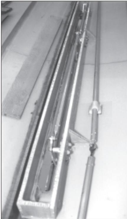
Honeycomb spoiler box, spoiler, and aileron linkage installed in the lower half of the wing. Note the carbon fibre shear web just to the left of the spoiler box.
