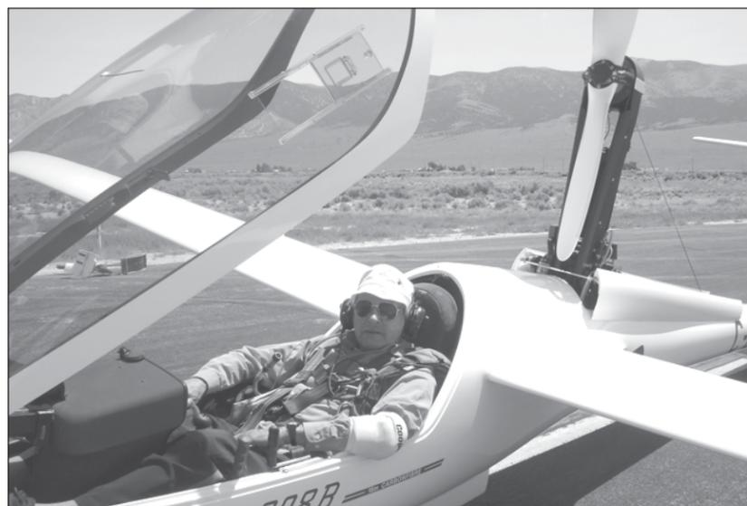
Here's Wilf in his DG808b motorglider prior to a launch in the USA. The prop is belt-driven from an engine that only partially extends out of the fuselage.
