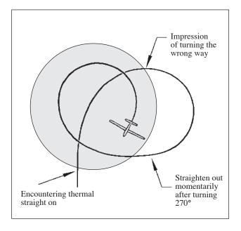
Don't make the mistake of tightening the turn when you are in the sink in an effort to expedite the process of getting back into the lift, if you hold the turn on a bit too long it may have the effect of centering in the sink. Simply maintain the same angle of bank till it's time to straighten out.
