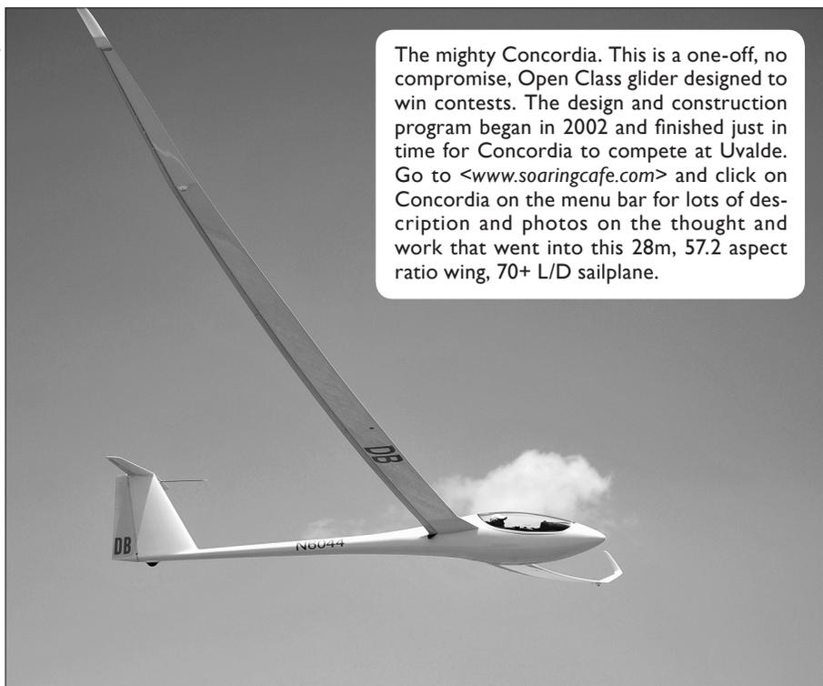
The mighty Concordia. This is a one-off, no compromise, Open Class glider designed to win contests. The design and construction program began in 2002 and finished just in time for Concordia to compete at Uvalde. Go to [www.soaringcafe.com](http://www.soaringcafe.com) and click on Concordia on the menu bar for lots of description and photos on the thought and work that went into this 28m, 57.2 aspect ratio wing, 70+ L/D sailplane.
