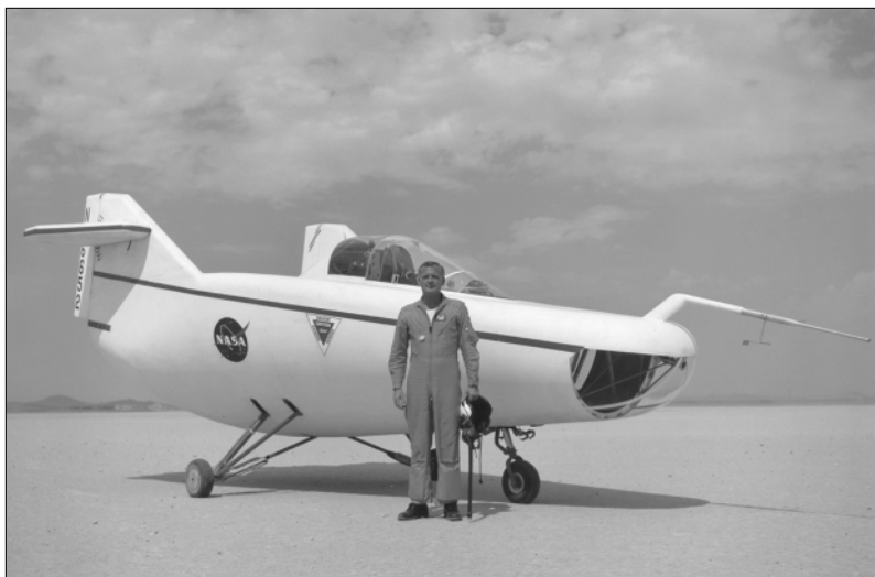
Milt Thompson and the “flying bathtub” on Edwards Dry Lake in 1963. Length 20 feet, height 10 feet, width 13 feet, weight (with pilot) 1140 lbs. photo: NASA-Dryden
