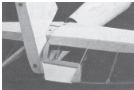
Elevator trim tab and other details of the tail feathers.
