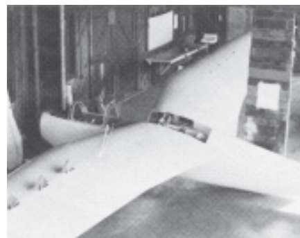
Nearing completion at Gatineau. Note the cut-back leading edge on the first 7 feet of the wing root — it's not a gull wing.
