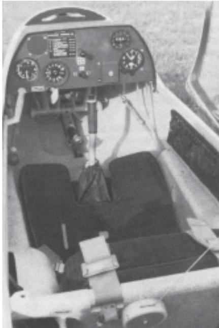
**View of the front cockpit. A neat touch is the reel stowage of the canopy safety cable just behind the front seat.**
