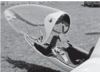
GLASFLÜGEL has recently been working on a project having the aim of completely redesigning the instrumentation and cockpit area of the modern sailplane. The company unveiled its "dream machine" which features a shallow cockpit pan cantilevered out from the main bulkhead, and a push-button instrument panel with all information appearing digitally on a "heads-up" transparent Liquid Crystal Display (LCD).
