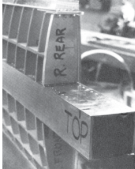
Dick Schreder's HP-20 wing structure in progress. Note foam ribs and large box spar which carries water ballast.
