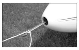
We found that a 14 mm wrench fit just right and stayed tightly hooked. A quick clove hitch around the wrench with the rope gave us what we needed, a secure way to tow the glider along the road and thus complete the *Metric Wrench Retrieve*.
