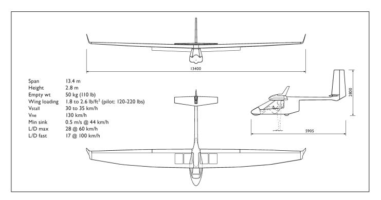
controlled by a lever located on the left hand side. There is very little load on the control column and the flaps add to the ease of flying and the glider's maneuverability. It may be foot or bungee launched off hills and winch, car, or air towed from the flat. It lands on a wheel and nose skid. The cockpit options can be open, partly-faired or completely enclosed.
