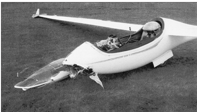
Modern brittle materials, such as the carbon fibre used in sailplane structures, have greatly increased static strength but inadequate impact performance.
