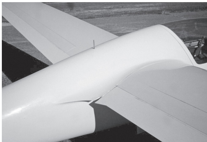
Straight TE tube permanently mounted on the Ventus fuselage top near wing drag spar bulkhead. It stands about 3 inches high, and performs well at that reduced height.
