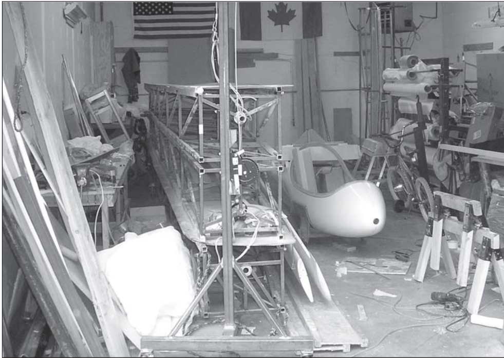
25 May 2008. Situation normal, all messed up. Foreground left, three of the four wing skin molds (fourth mold in other shop bay). Centre, the first-article fibreglass fuselage and canopy frame and assorted junk. Off to the right, materials racks. Background right, molds for horizontal stabilizer. Hidden right, molds for fuselage halves and for the wing spar.
