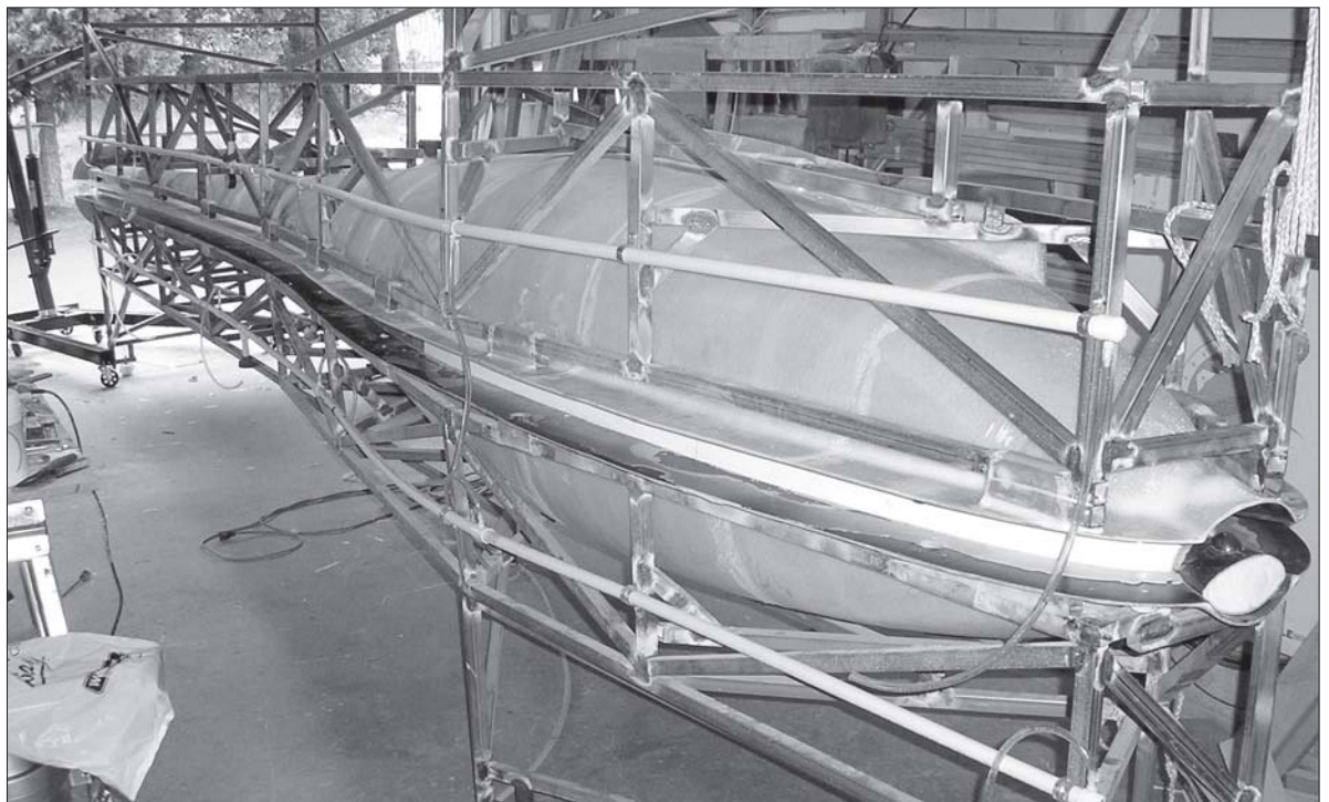
28 January 2006. The moment of anticipation as the heavily reinforced frame of the right hand side fuselage mold is being raised to release the first article fibreglass fuselage.
