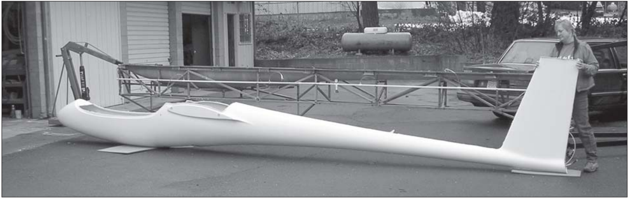
The first fibreglass fuselage, fresh from the mold.
