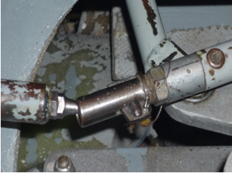
Standard L'Hotellier connection with locking pin
