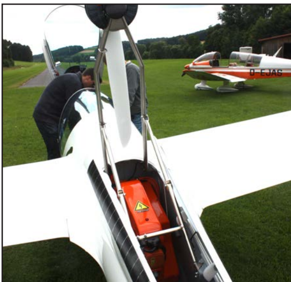
Picture 5 Location of battery pack in the front of the engine bay
