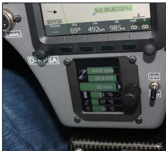
The engine instrument displays all relevant information
