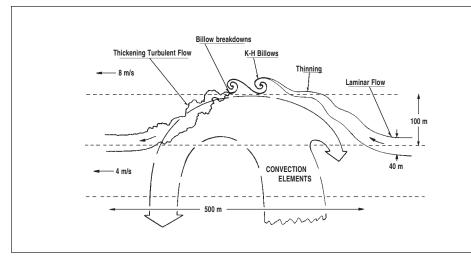
Fig. 5 (Payment and Readings, 1974): Schematic representation of a 'convection element' pushing into the nocturnal inversion, forming an 'inversion hummock' and entraining relatively warm air which is carried back down into the convection layer.
